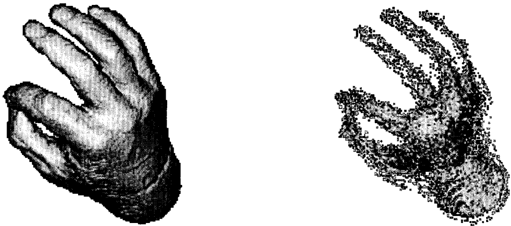
Fig. 5. To the left a hand. To the right a reduction of the hand using the 3-4-5 metric, containing 5.8% of the original voxels. (The copyright holders of this hand are Professors Jun-ichiro Toriwaki and Kazuhiro Katada, Nagoya University, Japan.)
