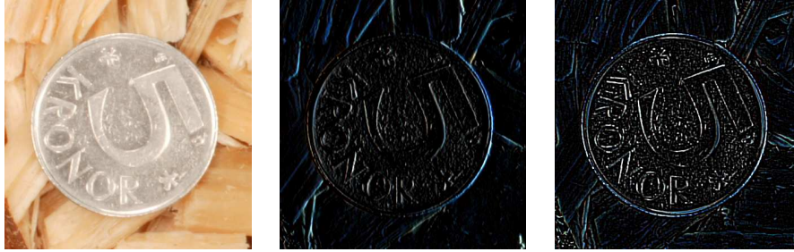
Figure 7: Original image (left), result after filtering with a vertical Sobel filter (middle) and result after filtering with a Laplace filter (right).
