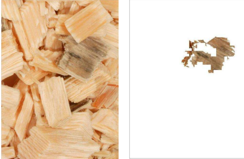
Figure 15: A bluish piece that is not bark (left), but identified as bark by the method (right).
