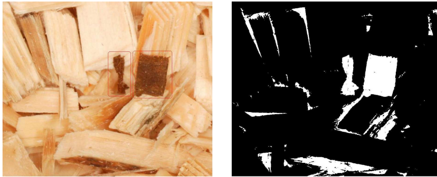
Figure 8: Original image with the bark marked with rectangles (left) and thresholded image (right).
