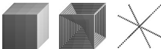
Fig. 4. A cube with its D^6 surface skeleton and the curve skeleton computed by our algorithm.
