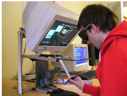
Fig. 1. The Reachin desktop display [10]. The PHANToM device [11] is positioned beneath a semi-transparent mirror. The graphics are projected through the mirror to obtain co-location of graphics and haptics.
