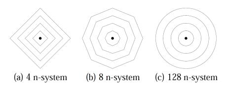
Figure 58: Distances in discrete grids [3]. The weight of each edge is equal to its Euclidean length.
