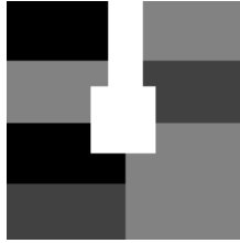
Figure 3: The custom tag design. 8 rectangular areas encode one of more than 6000 IDs using only three different grey values. The central white square is easy to detect, and the white line extending from it identifies the bee's orientation.
