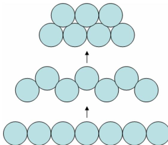
Fig. 1 The fibers in the flat topology (in the bottom) starts to climb on its neighbors (in the middle), creating a new topology and finally a flat topology is obtained (on the top) when the fibers have climbed as high as possible.
