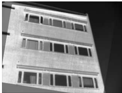
Figure 16: Registration result showing the fusion of thermal infrared and visible images by alpha blending.
