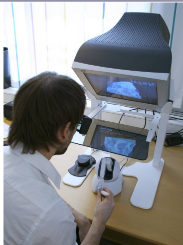
Figure 18: (Top) A user segments organs in a MR volume by placing seed-points representing organ and background, respectively. The segmentation is updated dynamically in real-time. (Bottom) A user working with the haptic display.
