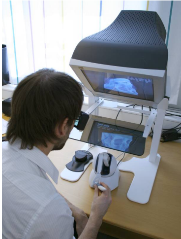
Figure 14: (Top) A user segments organs in a CT image by placing seed-points representing organ and background, respectively. The segmentation is updated dynamically in real-time. (Bottom left) A user working with the haptic display. (Bottom right) Final segmentation of a number of organs.
