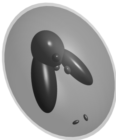
Figure 2: A three-dimensional version of the Shepp Logan phantom.
