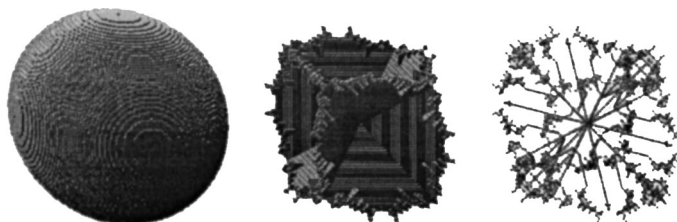
Fig. 12. A digital Euclidean sphere with radius 50 voxels (left), its surface skeleton (middle), and curve skeleton (right).
