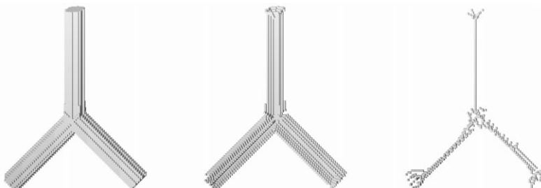
Fig. 14. Three fused cylinders (left), its surface skeleton (middle), and curve skeleton (right).
