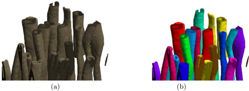
Fig. 6. Segmentation of fibres from the artificial volume with the proposed graph cut method. (A) The original volume from which lumen were segmented. (B): Each fibre is segmented, labeled and displayed.
